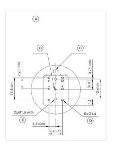
A = Drilling plan (component side)
